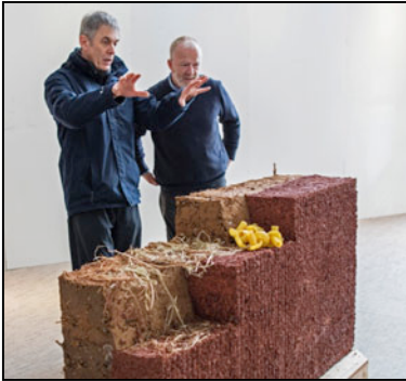
CobBauge test blocks
